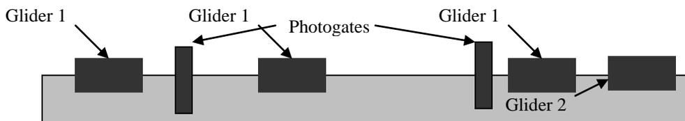
5. Set the photogates to measure the speed of the gliders. Each photogate should be ready to record up to two different speeds for each trial.
