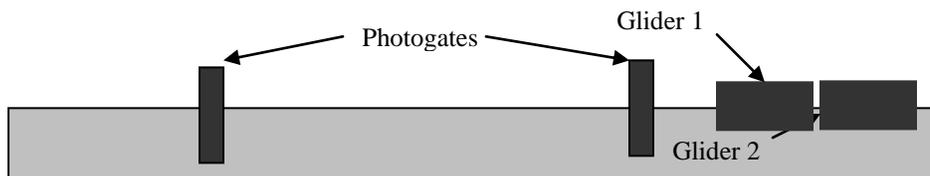
18. Set the photogates to measure the speed of the gliders. Each photogate should be ready to record up to two different speeds for each trial.
