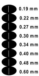
distances are between slit centers slit width = .084 mm
