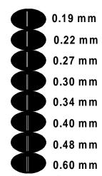
distances are between slit centers slit width = .084 mm
